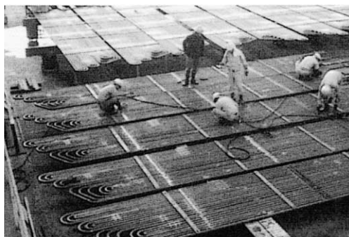
Photo 2. Fabrication of superheater tube bundles for steam boilers (Photo: Nagasaki Kogyosho Co., Ltd., Japan)
