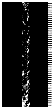
Fig.4 - An Example of Bead Profile of MX-100T in Welding Fillet Joints -Base Metal: 2.0-mm-Thick -Wire Size: 1.2mm4> -Welding Current: 80 A -Position: Vertical-Down
