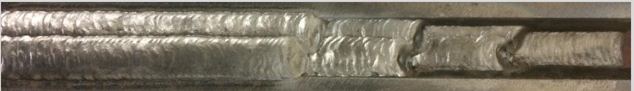
DW-50, 0.045", vertical upward welding at 64kJ/inch with mixed gas
