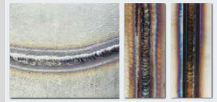
TG-X weld appearances without back purging: back bead (left/middle), face bead (right)
