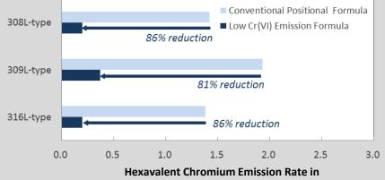
Welding at 200A with 75%Ar-25%CO<sub>2</sub> (mg/min)
