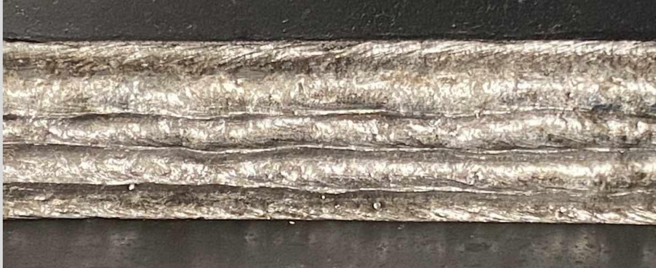
DW-50AY, 3/32", Horizontal Fillet Welding at 43.2kJ/in with 100%CO 2 gas
