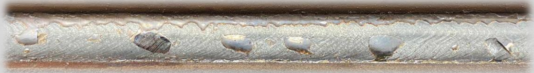
MX-A70C6LMn, 0.045", Horizontal Fillet Welding with 90%Ar+10%CO 2 mix gas
