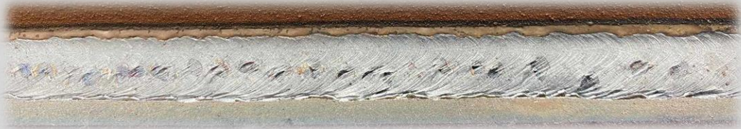
MX-A70C6SA, .045", Horizontal Fillet Welding with 75%Ar-25%CO 2 gas
